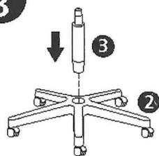
Place the 5 star base with the castors inserted onto the floor. Put the gas pump into the hole in the 5 star base.
