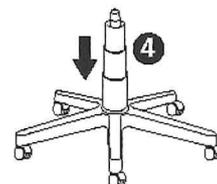
Push the plastic telescope all the way down so that it touches the 5 star base.
