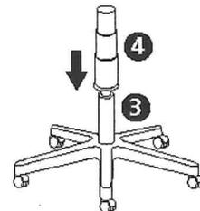
Place the plastic telescopic cover over the gas pump and push downwards.
